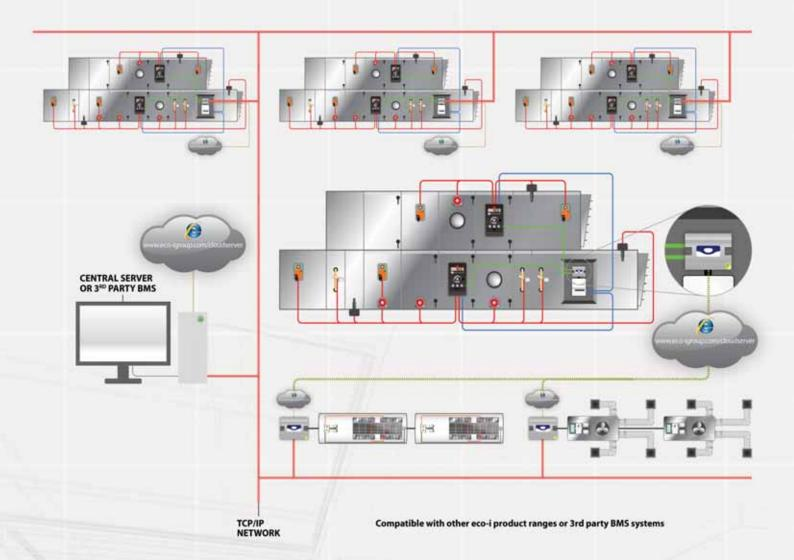
The inverter I/O is utilised to allow the most complicated of AHU arrangements to be controlled via the eco-i net. The BACnet interface exposes the full array of parameters held within the inverter device. Each unit can operate stand alone or part of a site wide BMS system.
